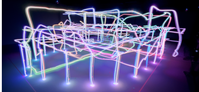
Fig. 1: Long exposure of 32 quadrotors navigating a cluttered environment.
